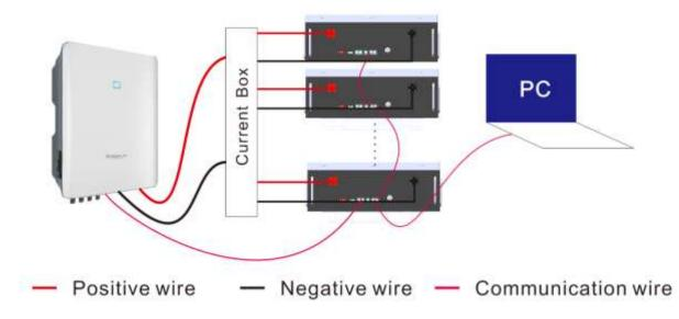
Note: RS485 communication address can not be 0, the address set by the host computer is required to be the same as the battery communication address, do not have duplicate addresses, otherwise communication may be affected.
